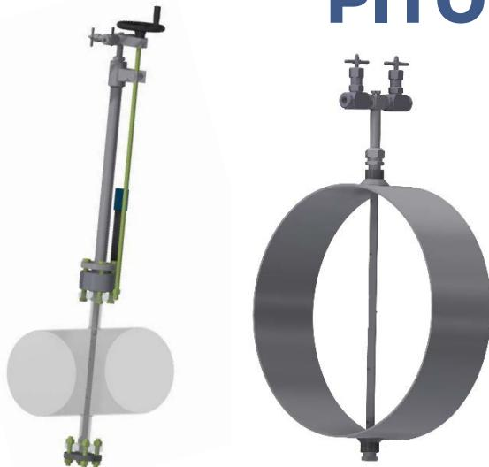
The Multiport Averaging Pitot Tube (Mapflow) is a differential pressure device suitable to measure the flow rate in a closed conduit for general applications (it is a general purpose and affordable device). Normally used in big pipes with low flow
